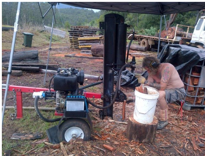
Timber splitting. This is a very labour intensive operation and is a productivity bottleneck
