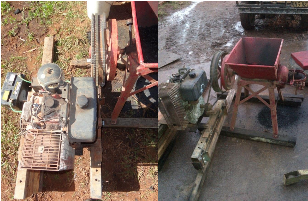
Grinder – Requires guard over belt drive and pulleys
