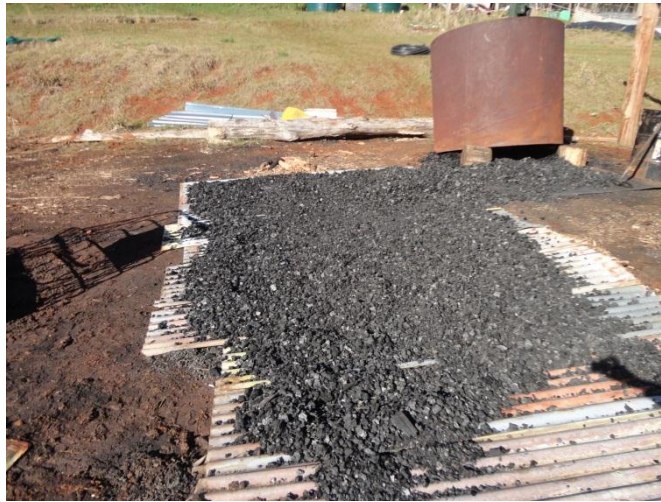
Product discharged onto metal sheets to reduce soil contamination risk.
