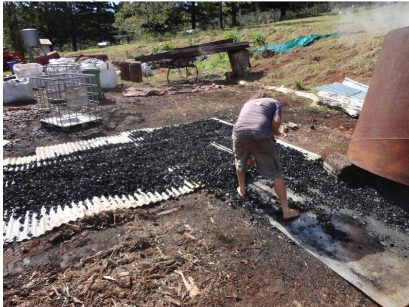
Product discharged onto metal sheets to reduce soil contamination risk.
