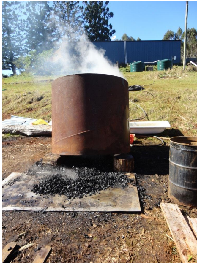
Char during discharge onto steel sheet to reduce risk of ground contamination
